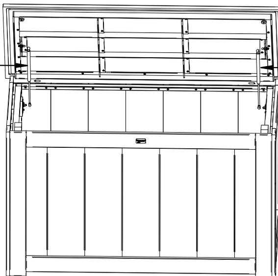
When attaching gas cylinders be sure to attach larger cylinder part to the top and smaller part to the base.
